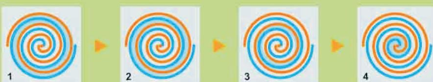
— Orbiting Scroll Rotor — Fixed Scroll Stator — Compression Room
